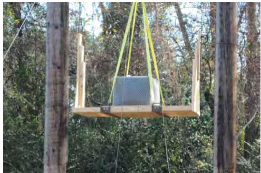
Figure 6 A Phase I Test Cube Being Raised on a Test Platform to a Height of 65 ft Prior to Drop Impact Testing
