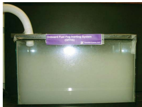
Figure 2: Lab tank filled with ultra fine kerosene fog
